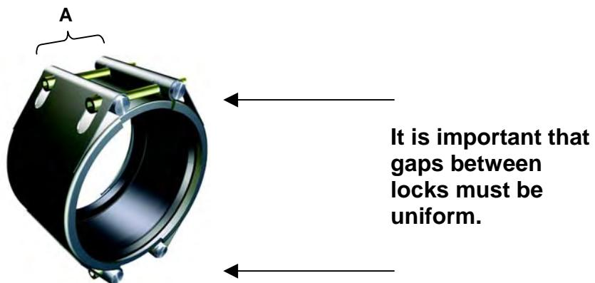
**ARPOL TRANS COUPLINGS ARE NOT DESIGNED TO SUPPORT THE PIPE OR TO PREVENT AXIAL MOVEMENTS. THEREFORE, THE PIPE MUST BE PROPERLY SUPPORTED AND ANCHORED.**
