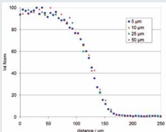
Fig. 5 Intensity distribution on a Mo knife edge for different step sizes
