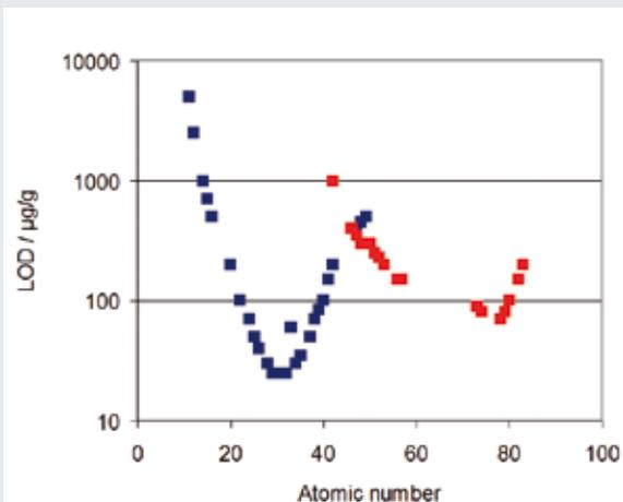
Fig. 6 Typical limits of detection for μ-XRF
