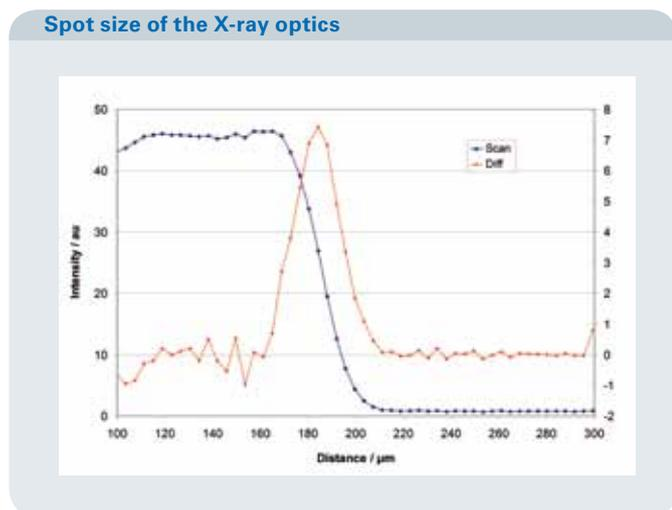
Fig. 1 Intensity distribution of a knife edge measurement for Mo-K and its derivative
