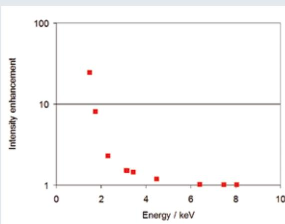
Fig. 8 Intensity enhancement due to measurement in vacuum
