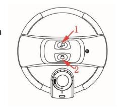
open the lid; press button 2, the lid will be locked to the pot and button will go up automatically.
