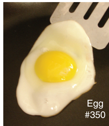
The Dry-Egg test under way on the new Eterna coating at Whitford's laboratory. All these eggs continued to lift easily off the dry surface of the pan, qualifying as a "5".
