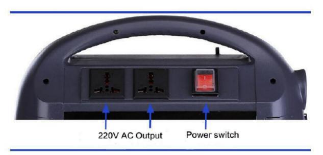
AC output: Both AC output sockets are with AC220V, 50HZ and output can be customized as 110V,60HZ output for Japanese and USA markets;  Power switch: Press it, AC 220V output will work, and the switch indicator lights; Press it again, output stops working and indicator is off.
