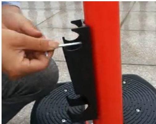
10. Stand on stepper to adjust two stepper to highest and lowest, then insert knob till final position. If not, computer can't show correct date.
