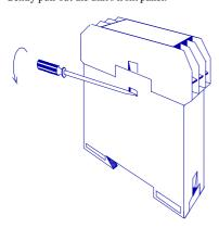
To close the unit, insert the printed circuit board in the proper side guiding slots and push it all the way until the front panel clicks with the body housing.
