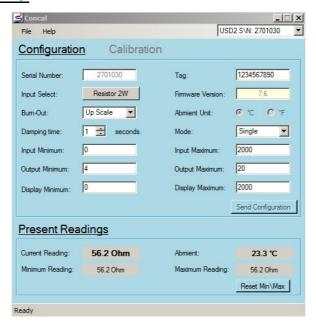
The main panel shows the connected unit's parameters, the configuration buttons and the current reading section.
