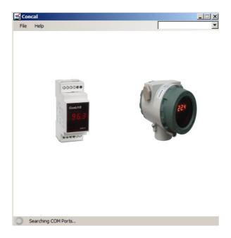
Connect the CON-USB cable to the PC and to the USD-2 unit. At the bottom line can be seen "Searching Com Port". It might take a while until the PC finds the proper COM port.
