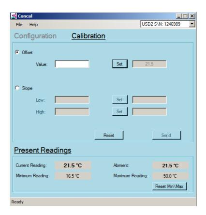
Calibration is a tool to compensate the sensor errors.
