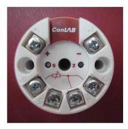
The RTR-2 is a non-isolated two-wire transmitter which converts the measuring signal of a platinum Pt-100 into standardized load-independent, 4-20mA current, linearly proportional to the measured temperature.
