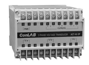
The ACT-4I3P and the ACT-4V3P isolated four-wire transducers accept AC current/voltage input signals and generate a proportional 4-20mA process output current.
