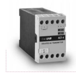
The ACT-4I and ACT-4V isolated four-wire transmitters accept ac current voltage input signals and generate a proportional 4-20mA process output current.
