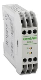
The DCI-2, a 2-wire isolated transmitter, accepts input voltage of up to 400Vdc or input current up to 100mA, generating a proportional 4-20mA process output current.
